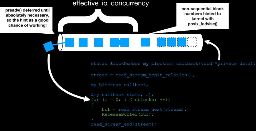
By issuing POSIX\_FADV\_WILLNEED as soon as possible and preadv() as late as possible, we get a sort of poor man's asynchronous I/O.
