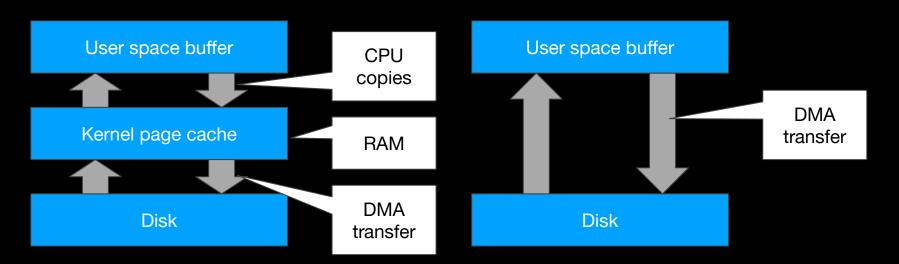
Direct I/O is an optimisation (CPU, RAM) and a pessimisation (when synchronous)!
